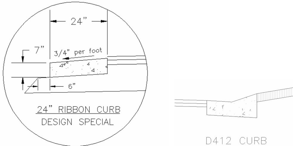
**Figure 6. Ribbon Curb Detail on the left and D412 curb on the right**
