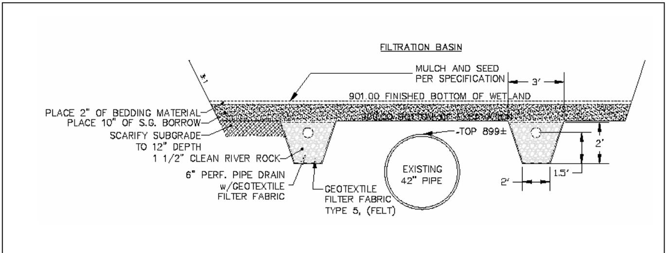
**Figure 7. Rainwater Garden Under Drain** (City of Maplewood, C.P. 02-10, 2003)
