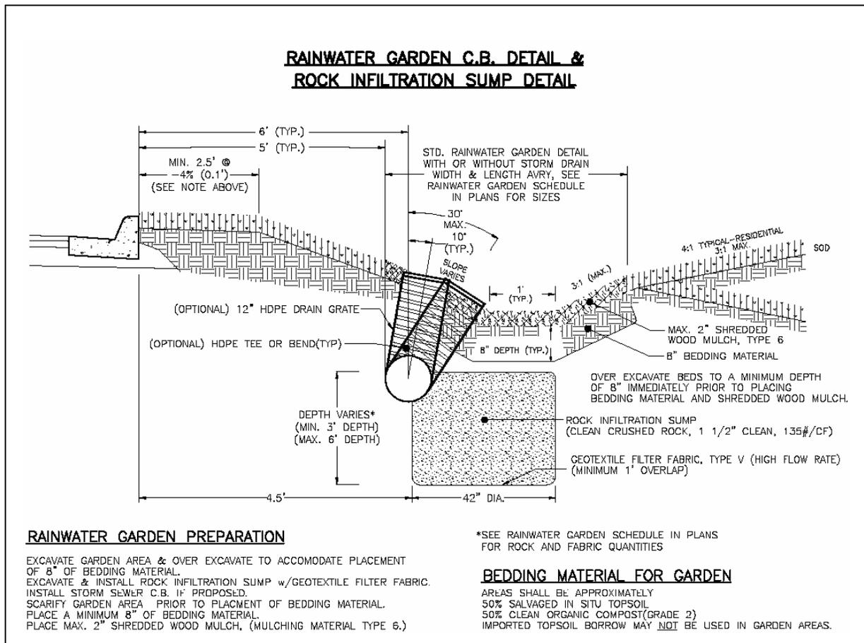
**Figure 1. Rainwater Garden Detail (City of Maplewood, Standard Plate 115, 2004)**
