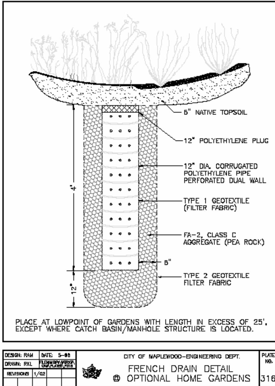
**Figure 2. French Drain Detail** (City of Maplewood, Standard Plate 316, 2004)
