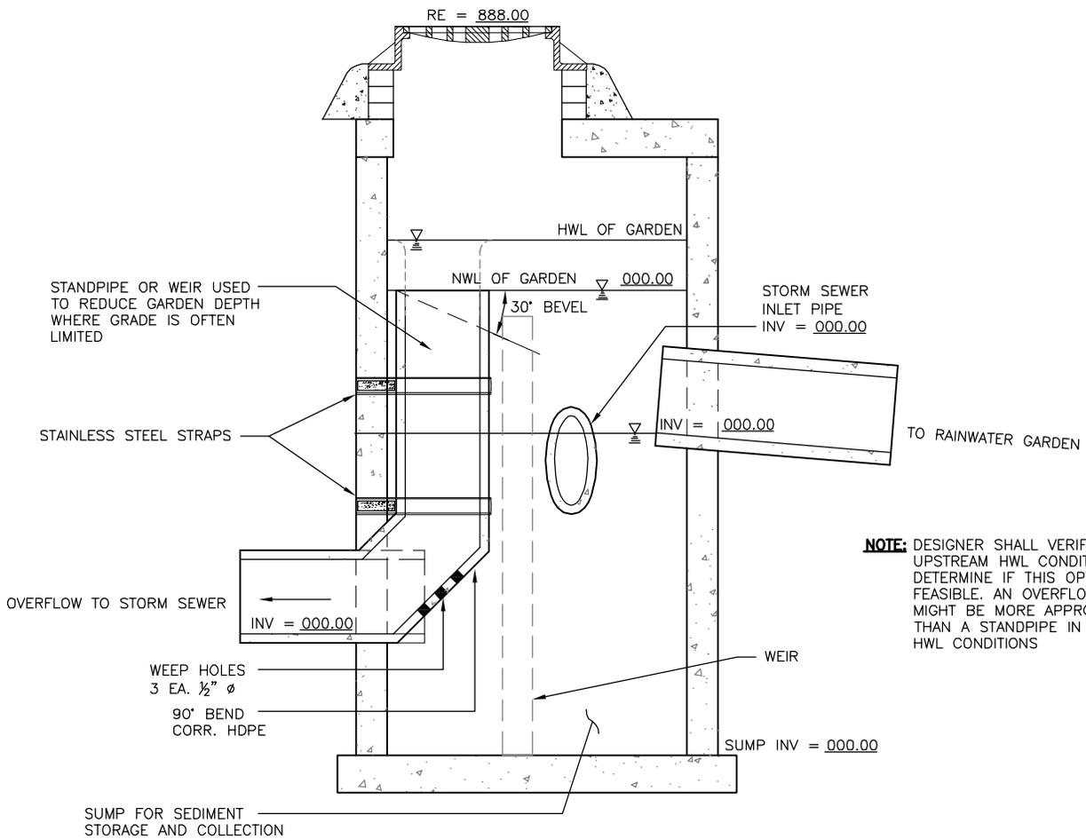
**NOTE:** DESIGNER SHALL VERIFY UPSTREAM HWL CONDITIONS TO DETERMINE IF THIS OPTION IS FEASIBLE. AN OVERFLOW WEIR MIGHT BE MORE APPROPRIATE THAN A STANDPIPE IN SOME HWL CONDITIONS
